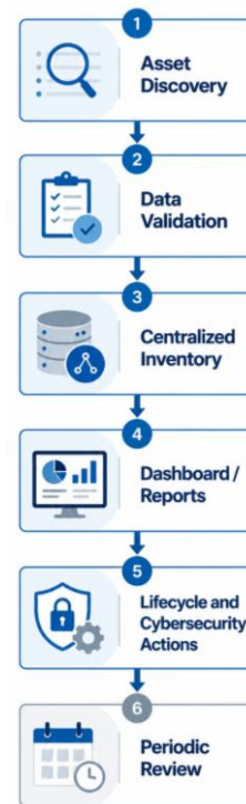
Figure 4 Future State OT Asset Management Process Flow Diagram
