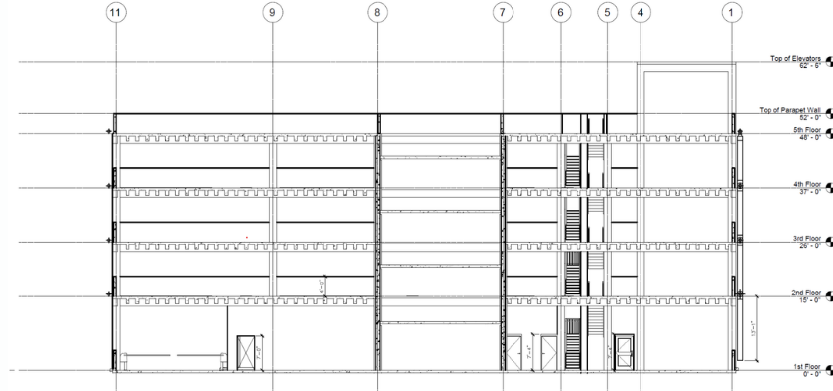
Figure 10: Multi-Level Structure Parking Elevation Section
