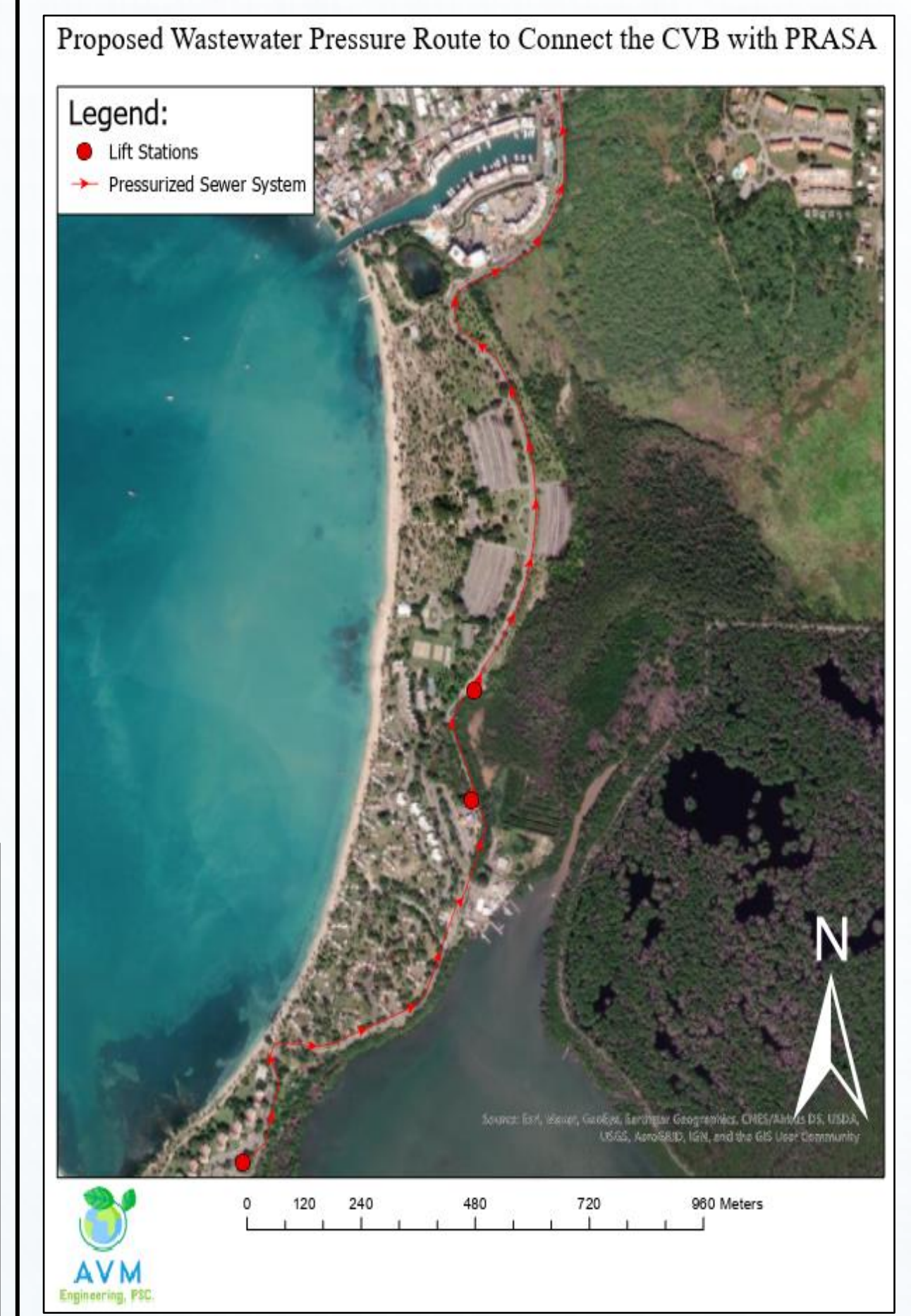
Figure 3: Proposed sanitary force line to connect the CVB to PRASA
