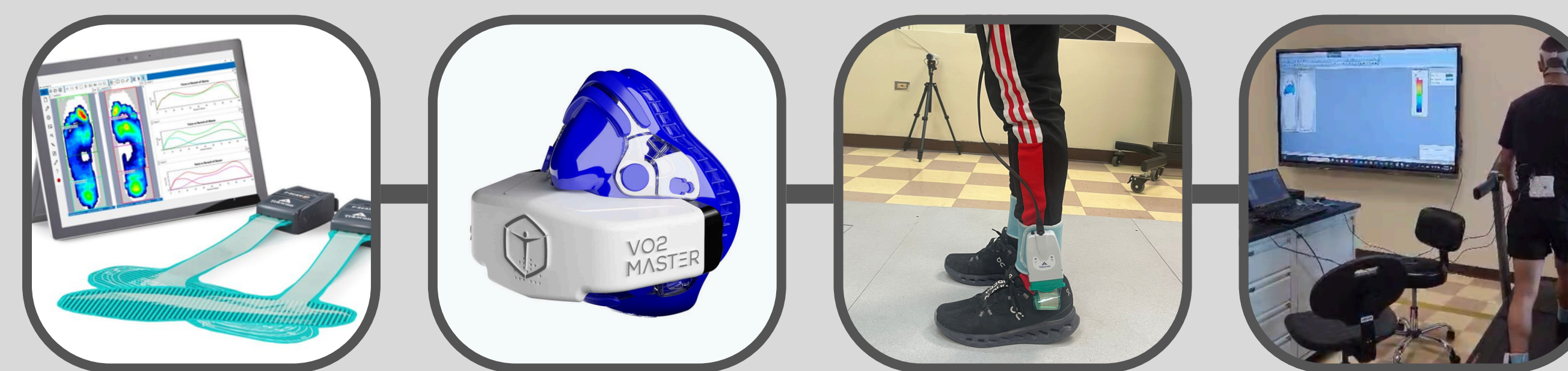
Figure 1. Equipment used for the research - Tekscan & VO 2 Master Metabolic Analyzer
