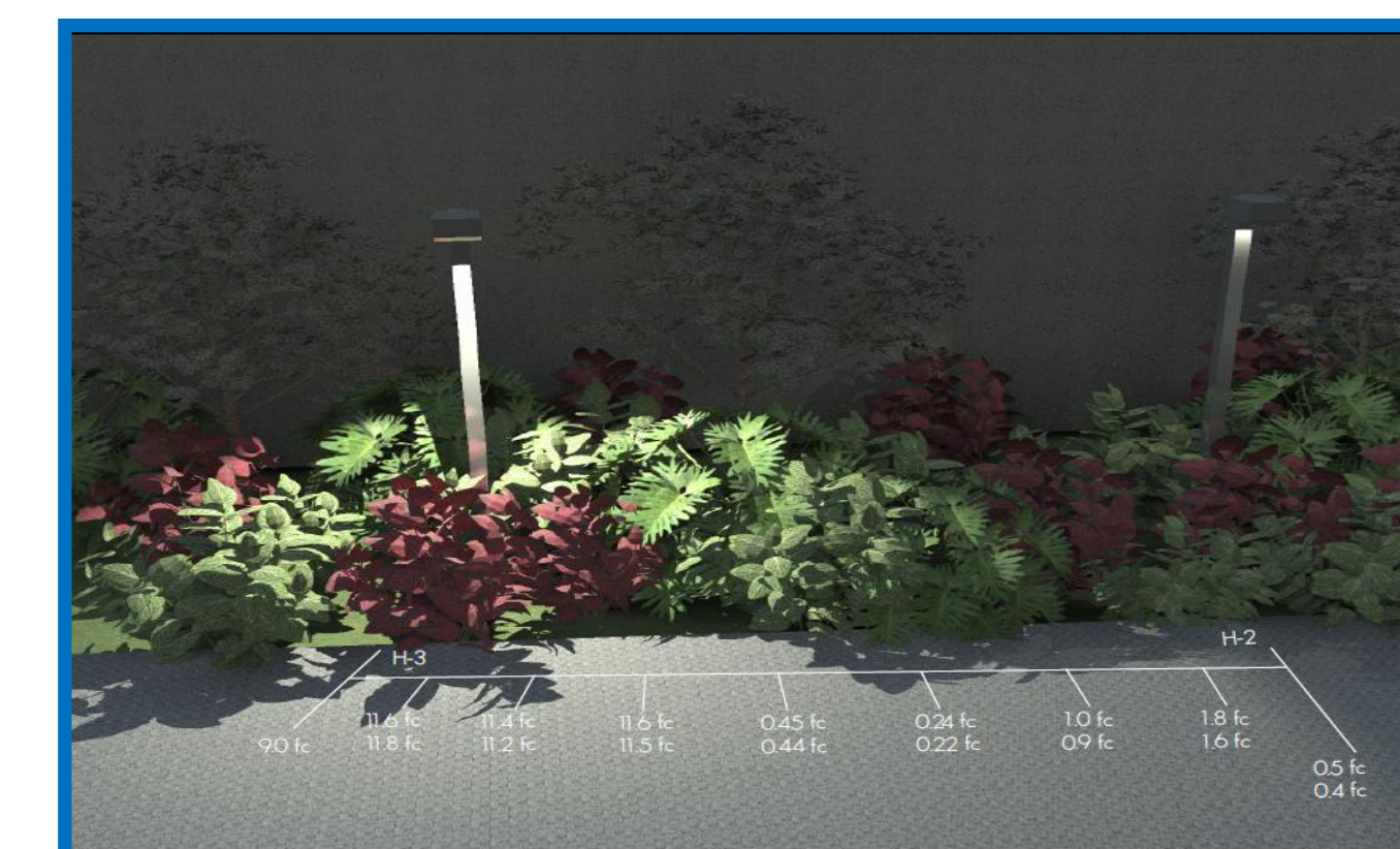
FIGURE 15: SCENARIO #2, INCONSISTENT ILLUMINATION LEVELS. SOURCE: FIELD DATA, MAY 2011.
