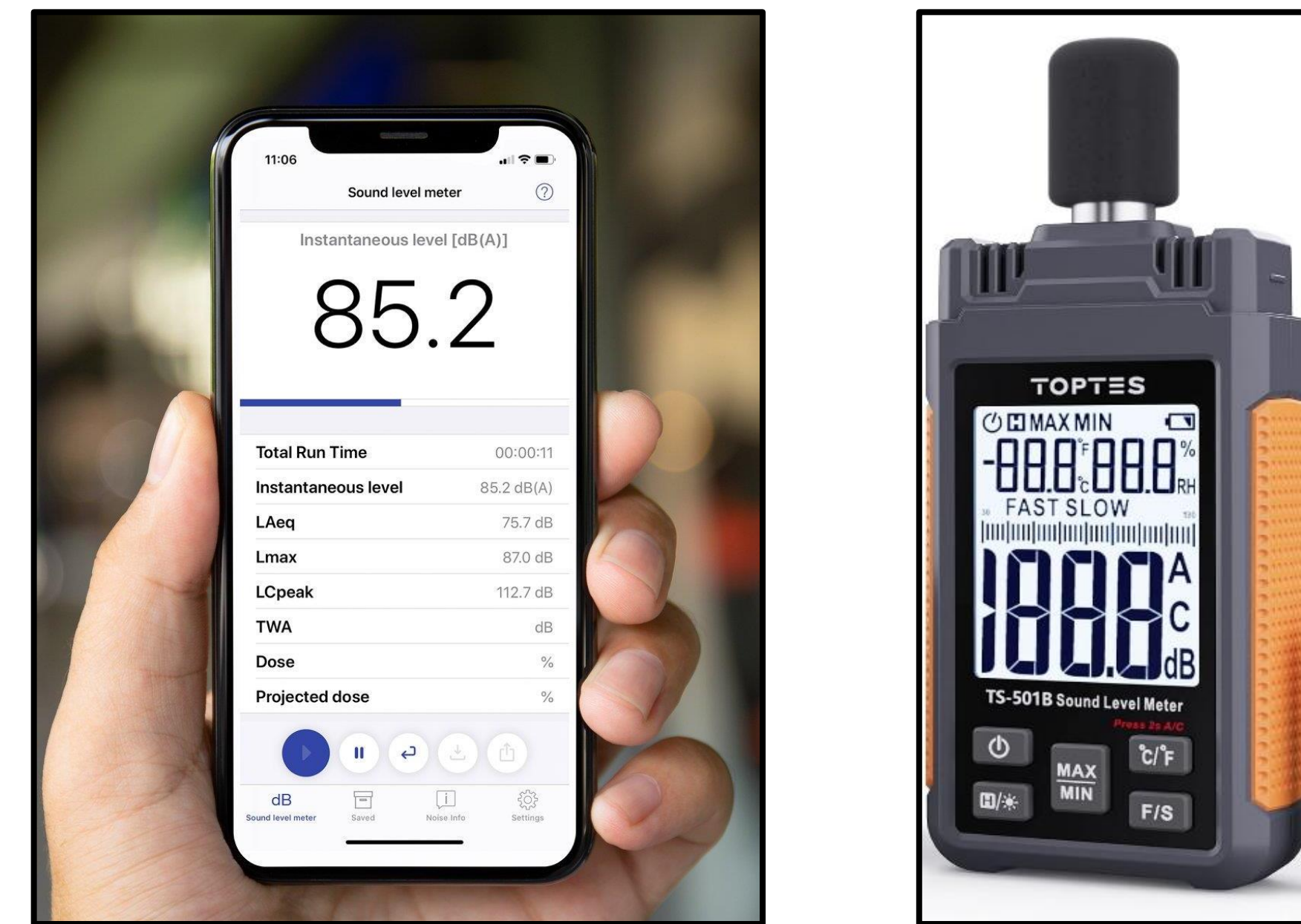
Figure 2: NIOSH Sound Level Meter App (Left side) & TOPTES Decibel Level Meter (Right side)
