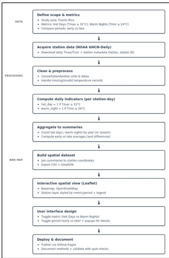
Figure 1 End-to-End Workflow for the Caribbean Heat Stress Atlas: Define Metrics, Acquire NOAA GHCN-Daily Station Data, Clean and Preprocess, Compute Daily Indicators, Aggregate to Annual Summaries, Build Spatial Datasets, and Deploy an Interactive Leaflet Web Map
