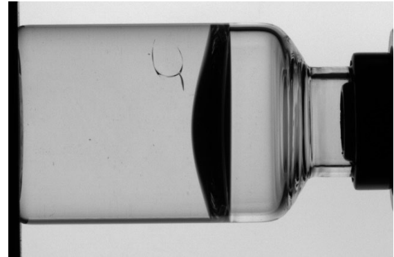
Figure 5 Crack Defect Insertion Using the Poisson Image Editing Technique
