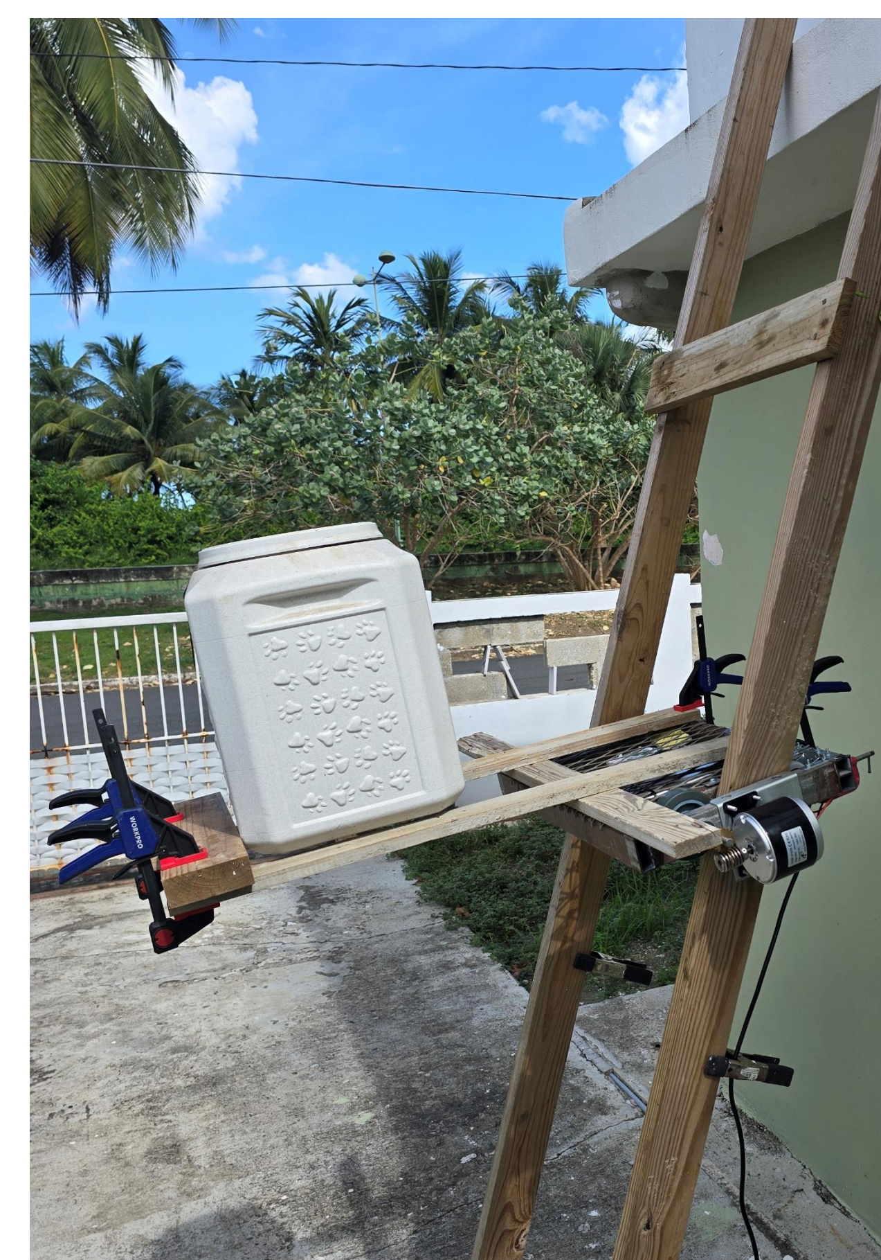
Figure 5 MLM prototype with 25 gallons of water approximately 200 lbs.
