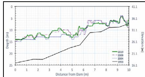
Figure 6 Bathymetric Profile of Lago Loíza for the Last Three Surveys and Compared to the 1953 Pre-impoundment Profile [7]
