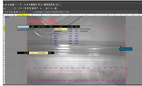
Figure 15 Product Under the Inspection Region & Sealed Area Partially Out
