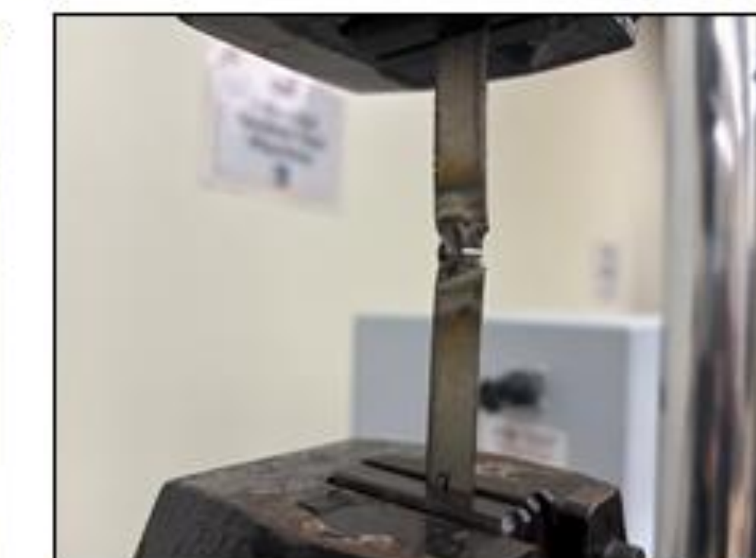
Figure 9 Close-up of Fractured TIG Weld Zone
