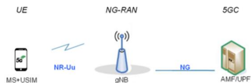
Figure 1 5G Network Architecture Components
