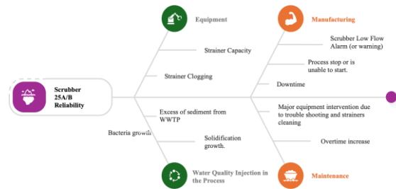
Figure 3 Fishbone Analysis to Evaluate Scrubber SC-25 A/B Issues Rule Out
