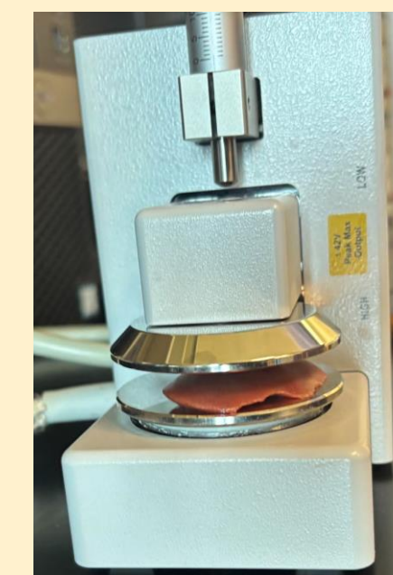
Figure 2: Keysight dielectric test fixture seen with electrode and kidney sample
