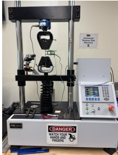
Figure 1 ATS Universal Tension Test Machine in the PUPR Mechanical Engineering Materials Laboratory
