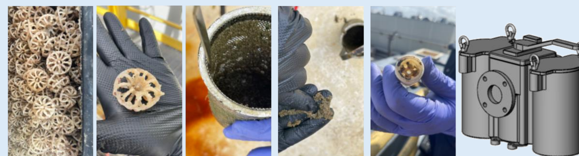
Figure 3 Solid Sludge and organisms trapped in packing and strainers
