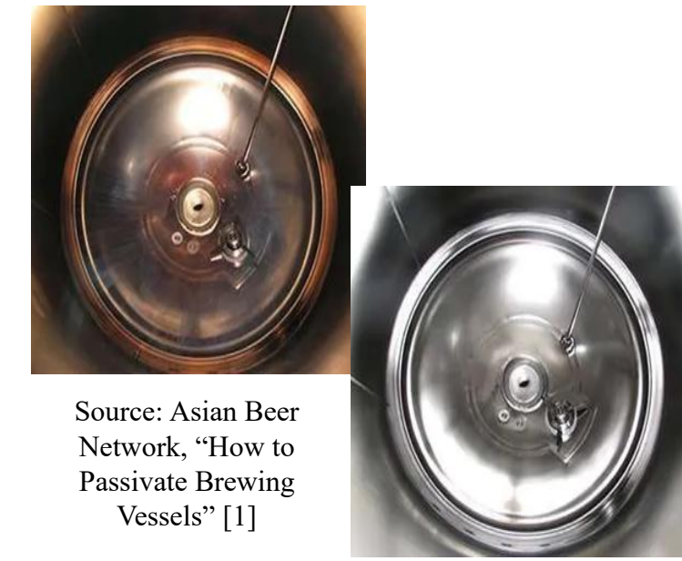
Figure 3 Before and after tank passivation
