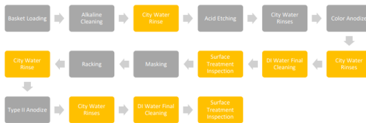
Figure 4 Proposed Process Flow for the Dual-Anodized Parts
