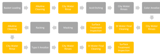
Figure 3 Dual-Anodize Flow
